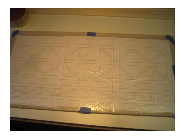
Both the horizontal stabilizer and elevator are constructed on the plans using just the supplied 1/4" thick balsa sticks cut to size, pinned and glued.
