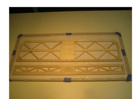
\*Transfer the center line of the horizontal stabilizer from the drawing onto the top surface of the stabilizer.
